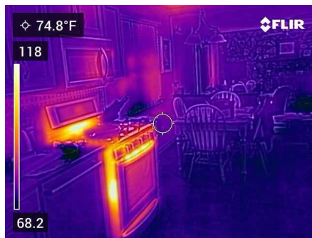
Thermal Image of oven operating
